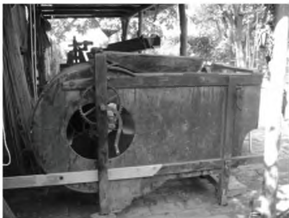
“Thresher” – a separator for the elimination of light particles from grains
